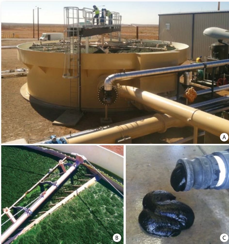
▲ Figure 7.2: Harvesting operations at large scale at Sapphire's Green Crude Farm, Columbus, NM, USA. (A) Harvest water from the ponds is sent to the Dissolved Air Flotation (DAF) unit. (B) Primary dewatering product. (C) Concentrated algae paste, ready for extraction or drying.
