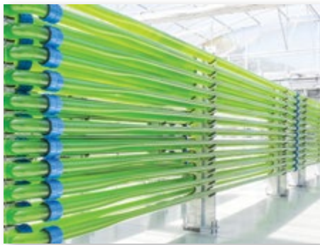
▲ Figure 7.3: Tubular fence photobioreactor with 10-m glass tubes
