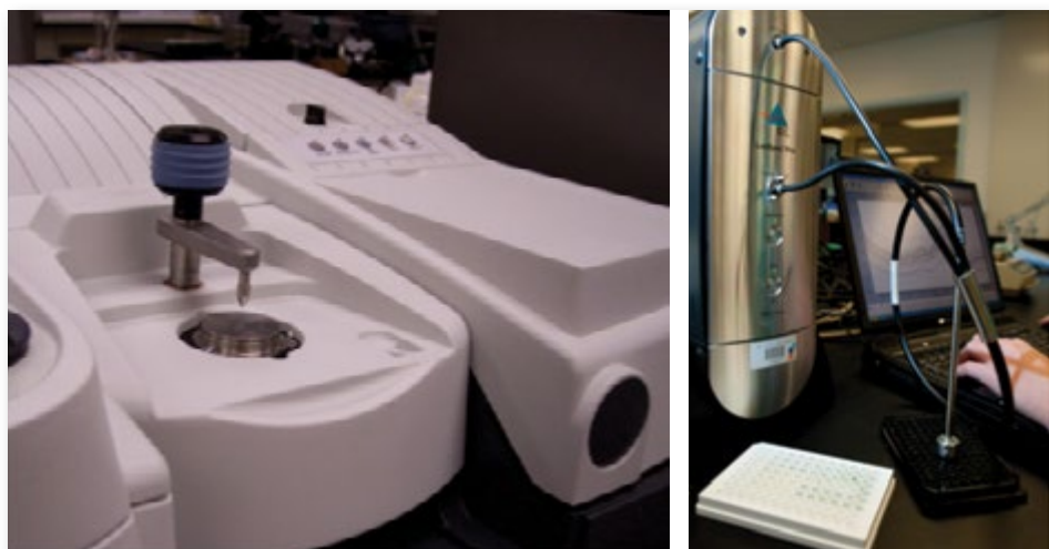
▲ Figure 1.2: Illustration of mid-infrared (left) and near-infrared (right) instrumentation for rapid spectroscopic fingerprinting of the biochemical composition of algal biomass
