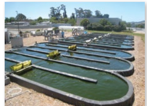
▲ Figure 4.1: Raceway ponds for wastewater treatment and algae biofuel feedstock production at Cal Poly State University, San Luis Obispo, US
