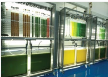
▲ Figure 7.4: Bubble column (top) and flat panel photobioreactor (bottom) at the Algal Research Laboratory at Arizona State University, Mesa, AZ, USA
